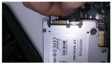
Now we must extract the screws that are subject to the SSD (all with a simple screwdriver for Phillips 1) keeping an order to use them in the newly acquired 1Tb SSD in the same positions. When you screw the ones located in the lower part of the images, do not tighten them completely.
