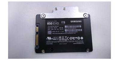
The following steps are like the previous ones but in the opposite direction, wiring connection (looking at the position of the connector that is L-shaped), insertion of the SSD in the chassis, relying on the chassis itself, fitting the pivots on the opposite side and finally tighten the screws that fit into the chassis. We replace the top cover of our Teknopack and the work will be done.
