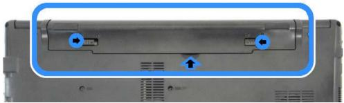
2.- While holding the latch in place, pull the battery up in the direction of the arrow and lift it out.
