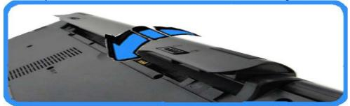
6.- Slide the latch in the direction of the arrow into the lock position.
