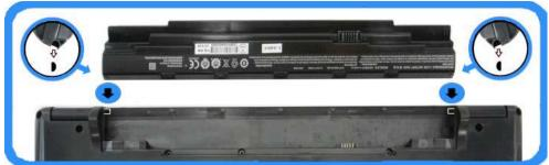
5.- Turn the battery in the direction of the arrow to insert it into the compartment.
